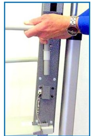
Remove Locking Pin Then Lift Handle Upward
