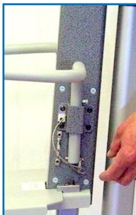
Remove Locking Pin Then Lift Handle Upward
