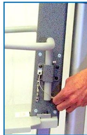
Remove Locking Pin Then Lift Handle Upward
